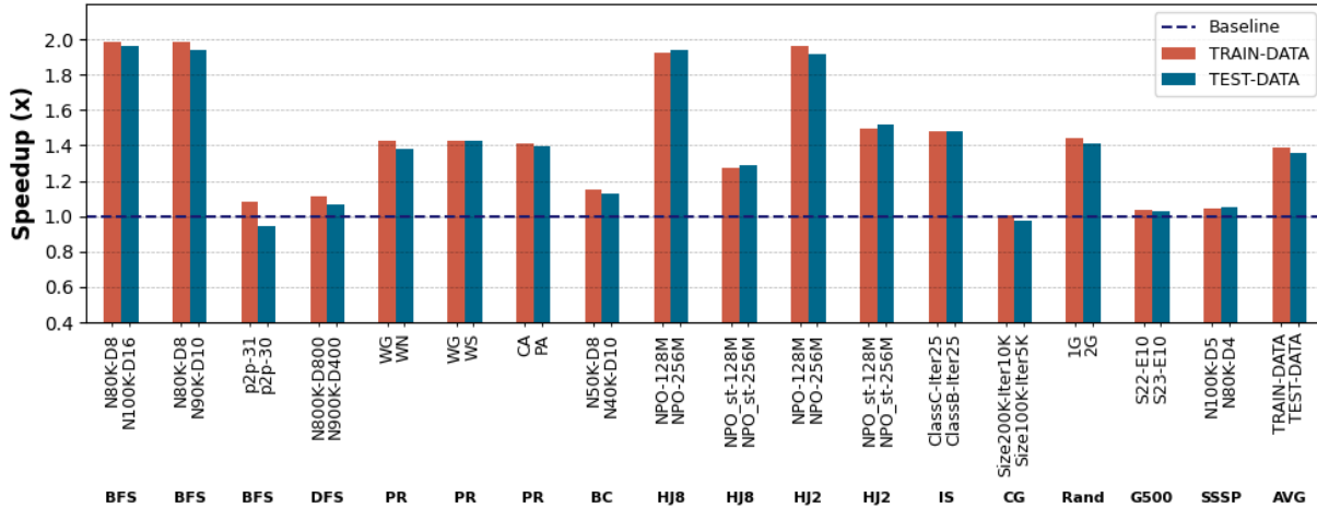
Figure 12. Execution time speedup provided by APT-GET over the non-prefetching baseline for different inputs as train/test data: APT-GET achieves 1.36\times average speedup on average for test data sets compared to the 1.39\times average speedup obtained for train data sets
